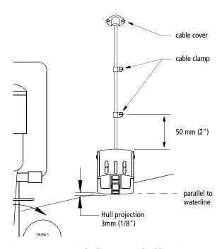
Figure 2-10: Vertical Adjustment and Cable Routing
